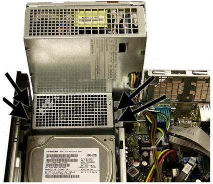
Figure 6-62 Removing the power supply
